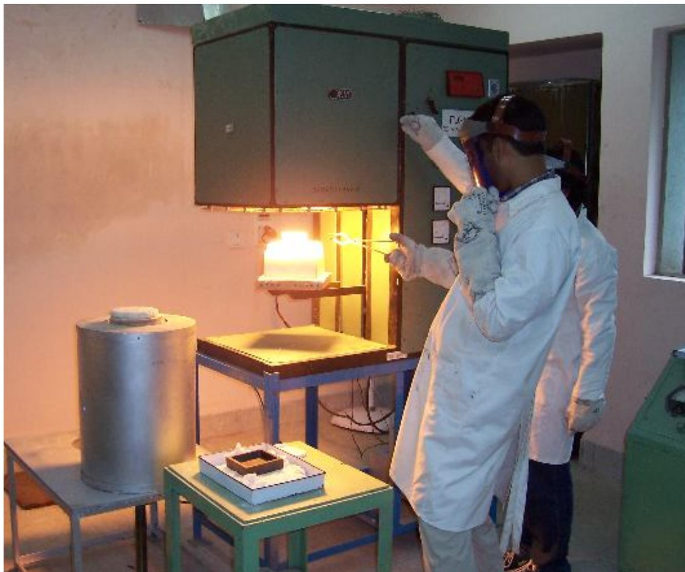
**Pouring of glass melt at  $1550^{\circ}\text{C}$  from a lowering and raising hearth type furnace and annealing at  $500^{\circ}\text{C}$**
